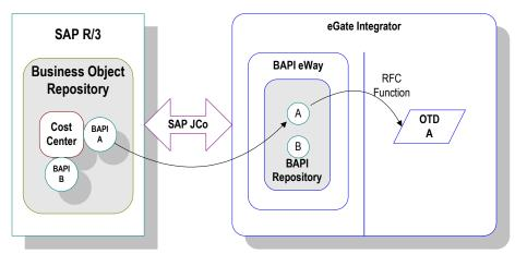
The functionality of the SAP BAPI eWay simplifies the process of determining the requisite **IMPORT**, **EXPORT**, **CHANGING**, and **TABLE** parameters—collecting all the necessary data using the correct type and format, calling the Remote Function Module (RFM) that represents the BAPI, and then extracting and parsing data from the **EXPORT** and/or **TABLE** parameters.
